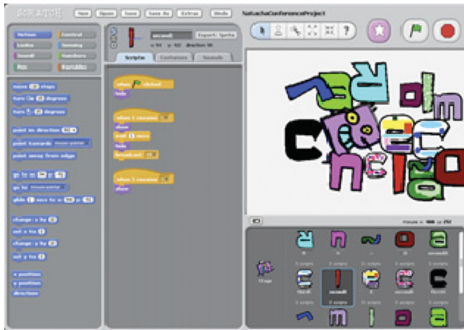
Fig. 1 Screenshot of the Scratch user interface. The leftmost portion of the screen lists available commands, the middle panel lists commands chosen to control the objects listed in the bottom-right panel, and the top-right panel is the design screen.
