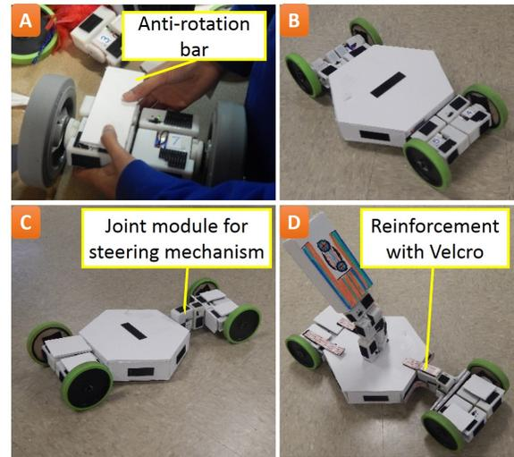
Figure 11. Learning by prototyping (a) Inserting anti-rotation bar to the two wheeled car (b) 4 wheeled car (c) 4 wheeled car with steering mechanism (d) Final 4 wheeled car with robotic arm
