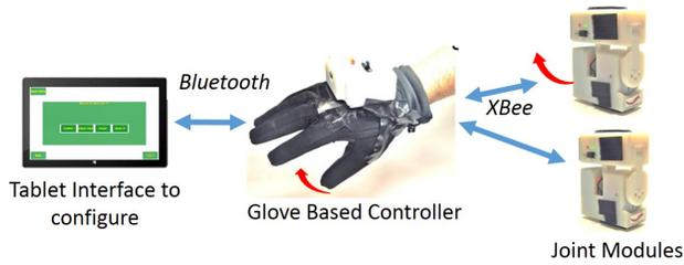
Figure 2. System overview showing flow of data
