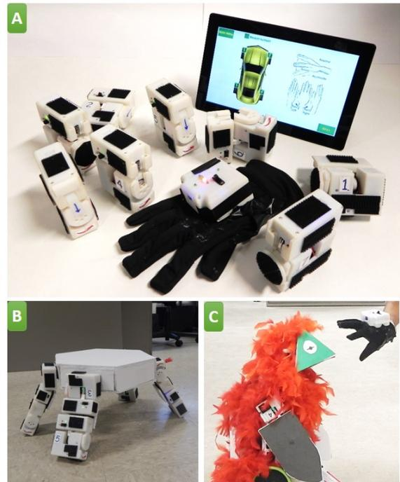
Figure 1. (a) HandiMate Kit (b) Sample creation (c) Gesture control of robot
