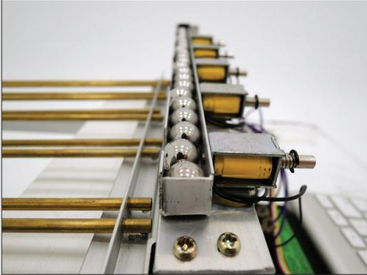
1 Electronic messages are encoded and transmitted mechanically via steel balls.
