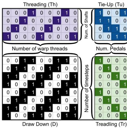
**Figure 2: A weaving draft for a typical shaft loom. Drafts describe how warp yarns connect to shafts (threading), how shafts connect to pedals (tie-up) and how pedals are actuated (treadingling) to create the weaving pattern (draw down).**
