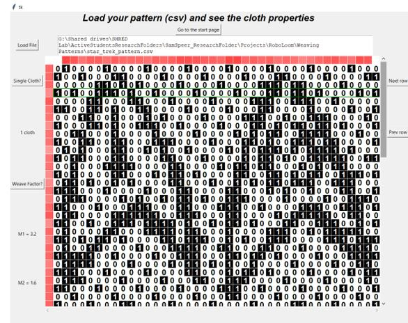
**Figure 6: SPEERLoom’s graphical user interface. The interface allows the user to load a pattern, visualize the cloth, explore the cloth properties by using the ‘Cloth Integrity’ and ‘Weave Factor’ buttons, and weave the cloth by using the ‘Next Row’ and ‘Previous Row’ buttons.**
